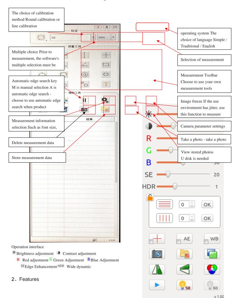
1) Camera Image Adjustment Settings: Drag the mouse to set the settings by clicking on the sliders, or click the sliders to set them with the mouse wheel.
