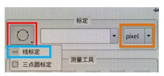
Press the round calibration icon on the top right corner, you can choose line or triangle calibration. Use line formed by 2 points for line for calibration, and use circle formed by 3 points for calibration. You can choose the correct way per the calibration type.
