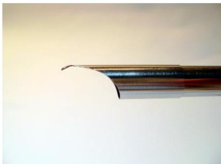
By using the curette user can look into tubing or tank to scratch the surface for rusting inspections. Put the curette on the top of the endoscope (see the left photo) and focus on the end of the small scoop.
