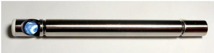
Reflector tube is used for side view of any tubing inspection.
