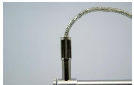
The endoscope can be moved up and down by turning the pillar (see left photo) for getting larger photo area or smaller photo area.
