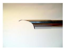
By using the curette user can look into tubing or tank to scratch the surface for rusting inspections. Put the curette on the top of the endoscope (see the left photo) and focus on the end of the small scoop.
