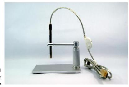
Plug the endoscope into the USB port, and double click on the icon of 'ehe.exe' to open the image window.
