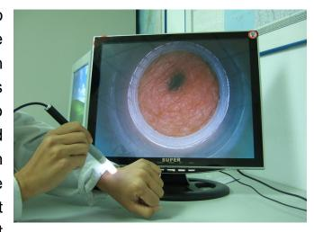
to view. You will always maintain a constant distance between the lens of the endoscope and the materials with this attachment.
