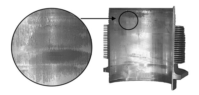
FIGURE 10 CYLINDER BARREL SCORING / PISTON RUB
