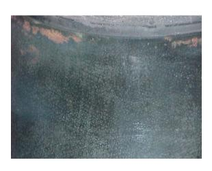
Phosphated cylinder bore. Note phosphate coating remaining in valleys of cylinder bore hone pattern. Light corrosion at top of cylinder bore, above piston ring travel limit. Presence of light corrosion in this area is normal.
