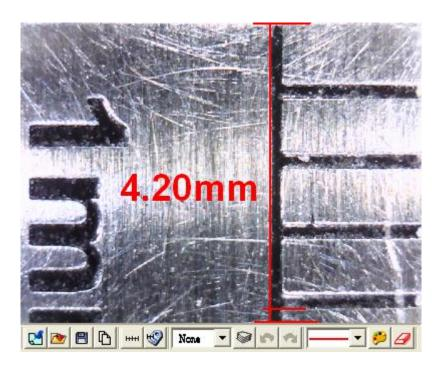
Fig. 5-36 vertical scale range is 4.20mm
