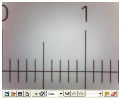
Fig. 5-41 horizontal scale range is 1.40mm
