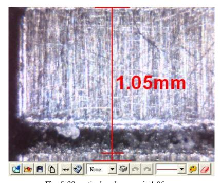
Fig. 5-38 vertical scale range is 1.05mm
