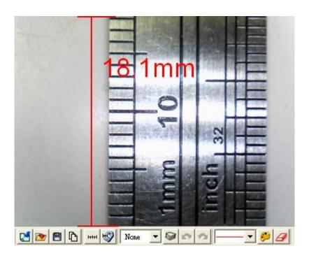
Fig. 5-34 vertical scale range is 18.1mm
