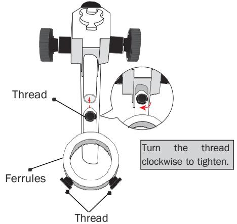
Step 3: Put the Wireless Microscope through the ferrules then tighten it clockwise with thread.
