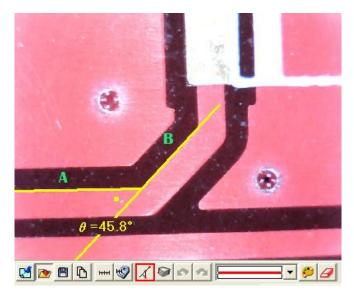
Fig 5-71 3 Points Chamfer
