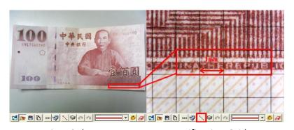
Fig 5-31b way to use Low Magnification Grid
