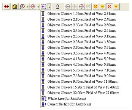
Fig 5-81 menu for Object lens 4x
