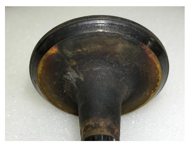
color, that does not continue from about 10:30 to 1:30 o'clock. The orange-ish color is likely missing from the top edge because the hot exhaust gases have burned it off that area as they escaped around the edge of the valve.
