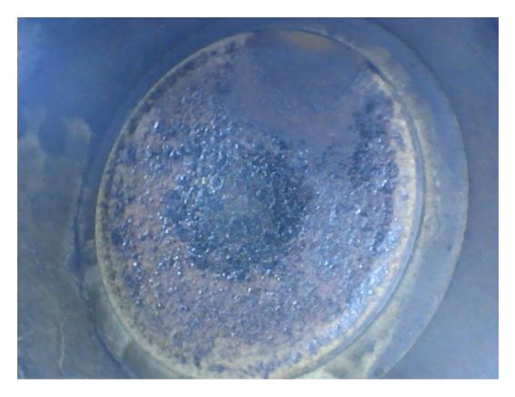
The upper right side of this valve (about 12 to 1 o'clock) shows a small hot spot, and the normal deposits have been burned off the surface.
