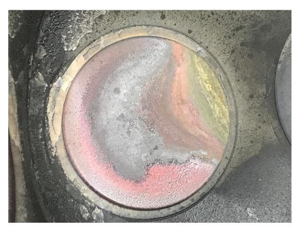
Here's the same exhaust valve, from a different angle after removing the cylinder. This one needed to go!
