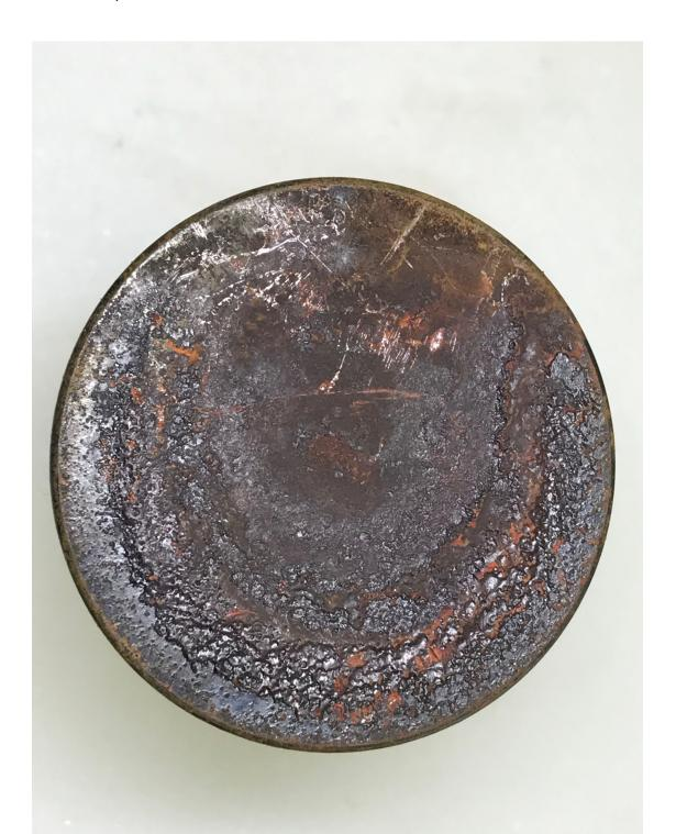
The trouble on this valve is at about 1 o'clock. Notice the smooth brownish area near the edge. The surface is smooth due to the deposits being burned off in that area.
