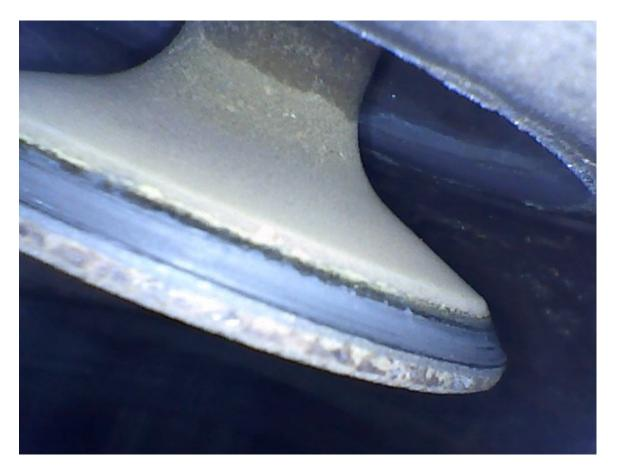
The valve grinding compound has restored a uniform band of sealing area both to the valve, and to the valve seat. It's hazy now, but over time as the engine runs, we're hopeful, a good, shiny seat will develop.
