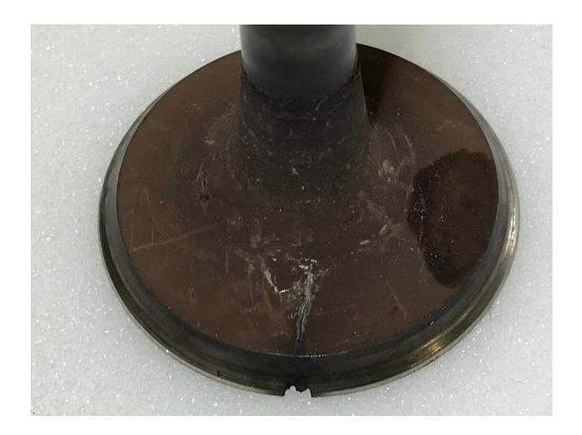
The previous picture shows how it was able to produce a compression test of 61/80... even though there is a chunk missing from the edge of the valve, there is still enough seating area left to make a seal.
