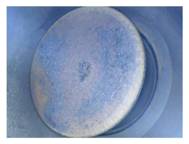
Notice the very small hot spot to the left from about 8 to 9:30. Also notice the distinct band of shiny area on the valve seat. It's consistent, but a little thin. I should have gotten a picture of the seat area over on the burning side.
