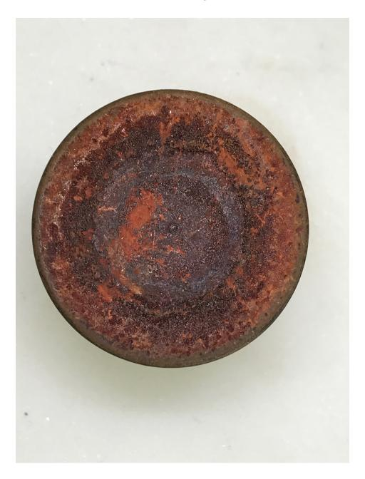
This is what you should hope to see when you look at your exhaust valves with a borescope. The reddish color is not a problem at all, and is totally normal. The concentric ring of deposits is an indication that all is well with this valve.
