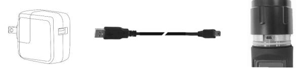
Connect one end of the USB lead to PC and the other end to the devices mini USB port , During charging the Power indicator will illuminate red,
